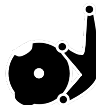
A Cam from a Babbage Analytical Engine
