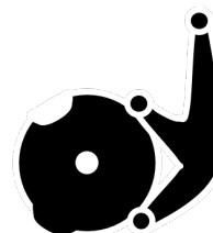
A Cam from a Babbage Analytical Engine
