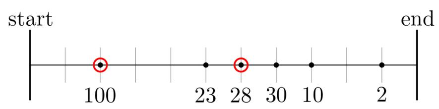
Figure K.1: Illustration of sample input. Metropolitan areas are depicted as points on the line. The optimal placement of stations is given in red circles, at distances 2.0 and 6.0 from the start of the line, with respective utility  $100$  and  $23 \cdot 1/2 + 28 \cdot 1 + 30 \cdot 1/2 + 10 \cdot 1/4 + 2 \cdot 1/16 = 57.125$ .
